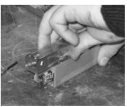
2. Slide the old reader head out of the scale housing and discard. Note the cable outlet direction as the new reader head cable will need to face in the same direction.
