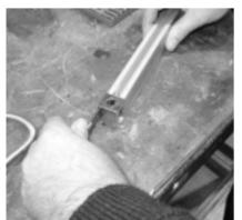
5. Push the mating parts together and replace the 4 screws in end plate Remove the excess salastic with a rag.
